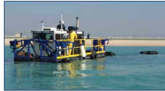
A Model 5012 LP removes silt from channels at a resort in the Middle East.
